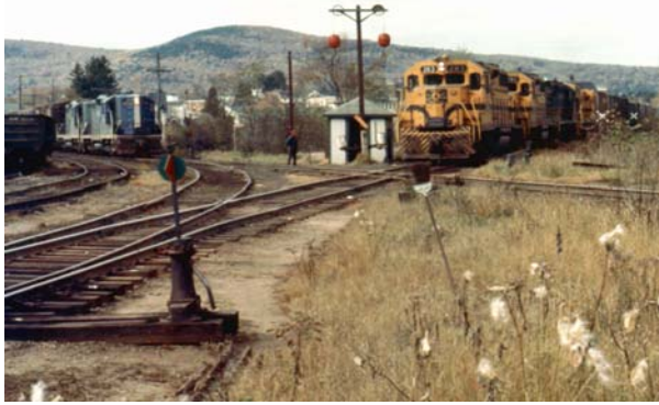
Figure 1 – 18 Maine Central train YR-1 at the “diamond” crossing of the Boston & Maine Railroad at Whitefield, New Hampshire. B&M train JU-1 (White River Jct. to Berlin) is off to the left. Note the ball signals to the left of the yellow Maine Central locomotive.
