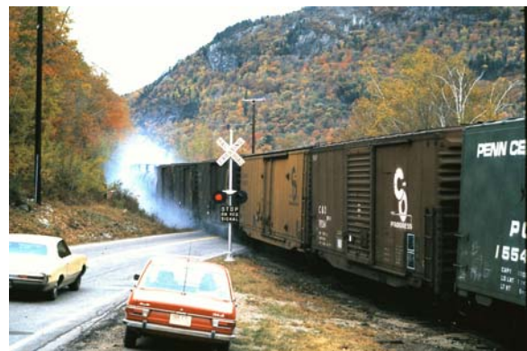
Figure 1 – 20 Heavy brake shoe smoke as down train YR-1 descends the Crawford Notch grade from the opposite direction of above photo.
