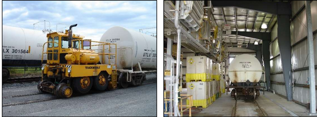
Figure 9: Trackmobile and Rail Car Transfer Facility 67
